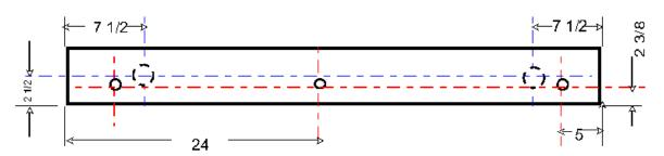
Drill holes at distances shown. If you use a spade bit, drill from both sides to avoid splitting the wood.
