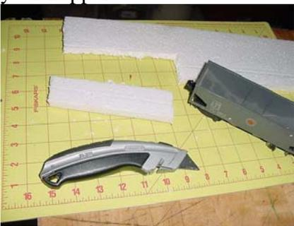
STEP 2 - Shape the Styrofoam with a rough file or, as in the picture, a Stanley Surform. Be sure to do this over a trash can.
