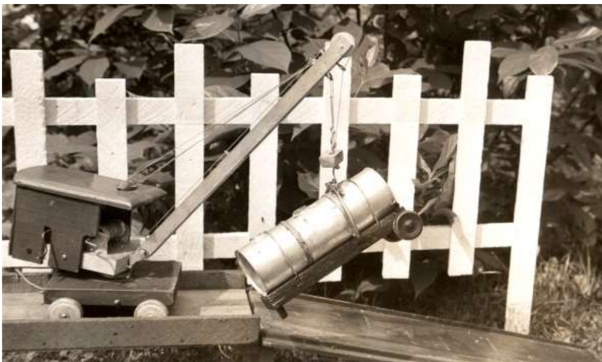
Roller skate wheels were used on the cab.
